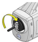
Mount the emitter assembly
